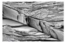
Since Mica has high aspect ratio it is widely used in plastic, polymer and phenolic compounds with electrical applications as filler of choice.
